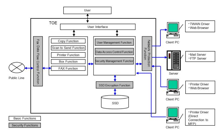
Please see section 1.4.3 in the [ST] for a more detailed description of the functionality shown in the diagram. There is no interface for any user or administrator to directly interact with the TOE operating system, all interactions must be made via one of the standard application functions or the hardware interfaces of the TOE.
